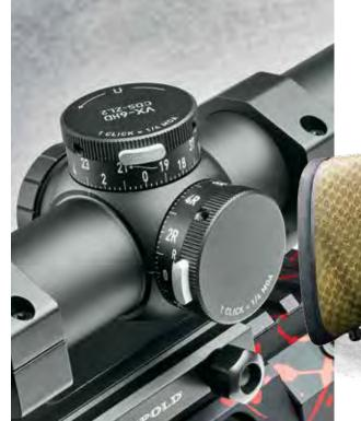
The CDS-ZL2 (ZeroLock 2) dial lock-release buttons partially retract when you reach the second revolution of adjustments, providing a visual and tactile indicator of your travel.
