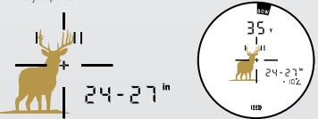
The benchmark settings here are 24 to 27 inches, and the whitetail being ranged is closer to the 24-inch mark. The hashmarks automatically adjust based on the range; in this case, 35 yards.
